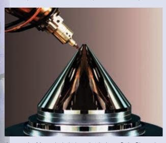
An example of the aspherical mirrors that the Large Optics Diamond Turning Machine first produced.
